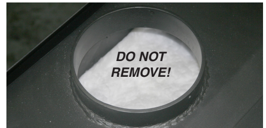
Figure 1 – DO NOT remove ceramic blanket from inside stove pipe opening. This is NOT packing material but an integral component of the stove combustion system.
