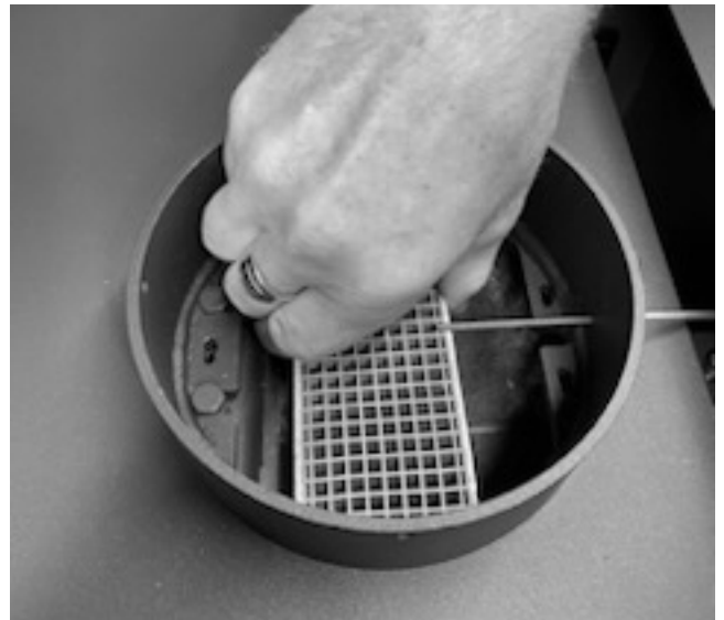
Figure 5: Position over combustor bracket.
