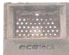
Basket needing cleaning with the holes blocked by ashes
