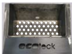
Clean burnpot with all the holes clearly visible
