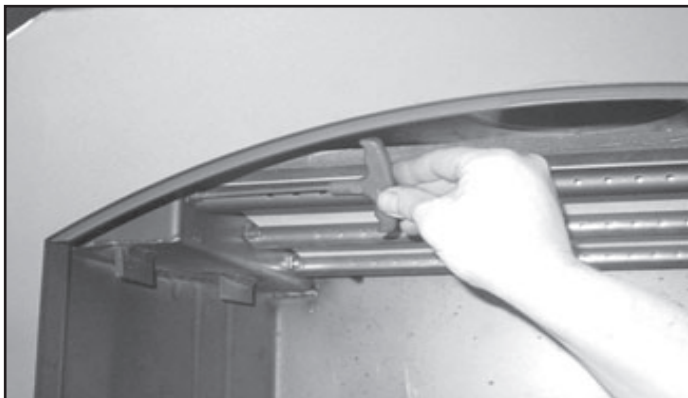
Figure 4.6 Removing Manifold Tube
