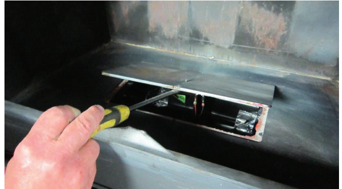
Figure 4.11 Open Access Door
