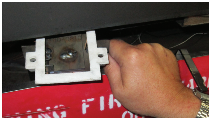
Figure 4.17 Inserting Timer Assembly With Gasket
