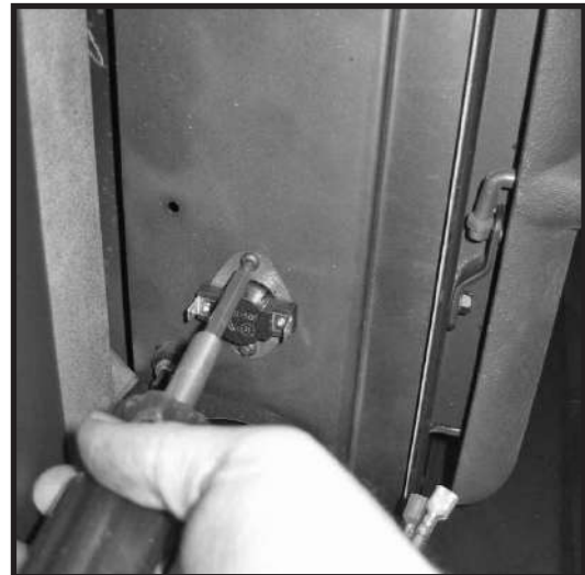
Figure 23: Relocating thermal switch to left side.
