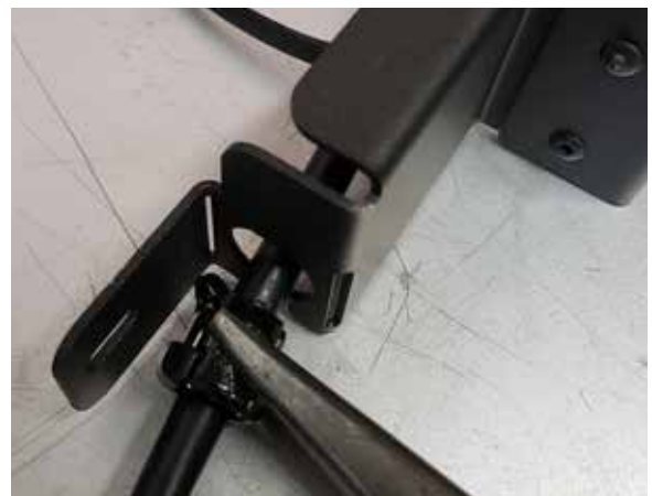
Figure 18: Left Strain install.
