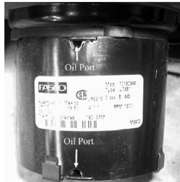
Figure 19. Oil ports on a circulation fan
