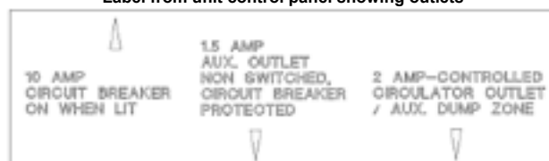
Label from unit control panel showing outlets
