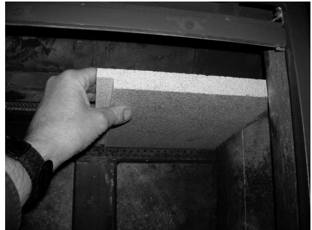
Figure 20 (cont.) - Removing/Replacing the Baffle for Inspection
