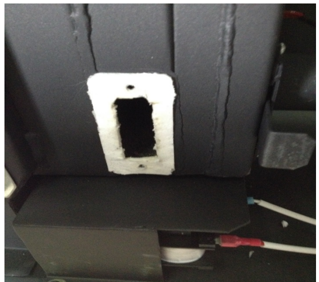
Figure 36: Remove lower exhaust chamber's cover plate and clean
