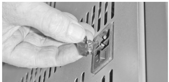
Figure 20b: Main power switch
