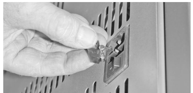
Figure 20b: Main power switch
