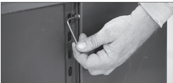
Figure 36: Remove side panel screws using 1/8 allen wrench
