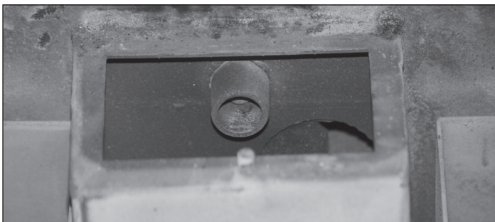
Figure 35: Remove ash from ignitor tube (underneath firepot)
