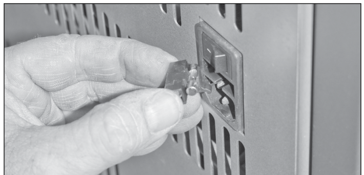
Figure 20b: Main power switch
