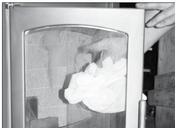
Figure 15: Wipe glass and inspect gasket
