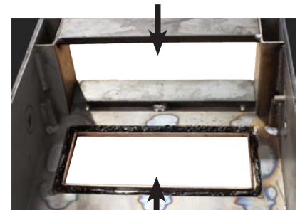
BYPASS DOOR OPENING
