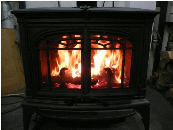
With the bypass and air control open, light the newspaper and partially close the doors (leave the doors open 1/4" for the first 2 to 3 minutes of startup).
