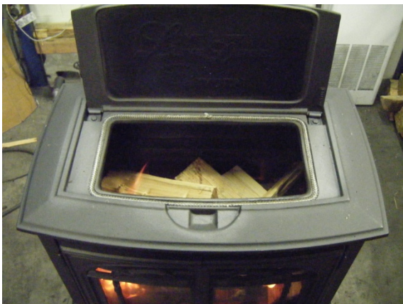
The 10 to 15 pieces of medium size wood will fill the stove approximately 3/4 full. The reason for using medium size pieces of wood is to acquire a coal bed as soon as possible.
