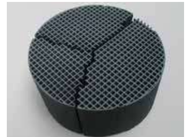
Photo #3 Thermal Cracks
