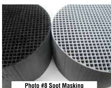
Photo #8 Soot Masking
