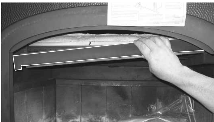
Figure 4.8 Removing Baffle Protection Channel
